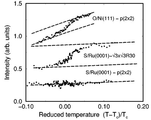
FIG. 2. Temperature dependence of the background intensity of the systems  $S/Ru(0001)$ - $p(2 \times 2)$  and  $-(\sqrt{3} \times \sqrt{3})R30^\circ$ , and of  $O/Ni(111)$ - $p(2 \times 2)$ , showing a characteristic increase due to uncorrelated site changes close to the respective order-disorder phase transitions. The dashed lines correspond to the increase due to thermal diffuse scattering alone. Curves have been shifted for clarity.
