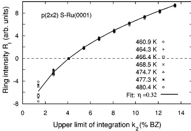
FIG. 14. Integrated ring intensities as a function of  $\Delta k_{\parallel}$ , for the system  $p(2 \times 2)$ -S/Ru(0001), and for the temperatures indicated. Again, data were taken both below and above  $T_c$  ( $T_c = 471.1$  K). Line: Fit to a power law according to Eq. (2).
