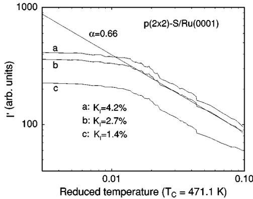
FIG. 5. Log-log plots of temperature derivatives of integrated intensities of superstructure beams as a function of reduced temperature for  $p(2\times 2)$  S/Ru(0001) below  $T_c$ , and for the radii of integration as indicated. The straight line corresponds to a power law with  $\alpha=0.66$ .
