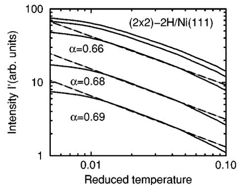
FIG. 4. Log-log plot of temperature derivatives,  $I'$ , of integrated intensities of first-order superstructure beams as a function of reduced temperature for  $(2 \times 2)$ -2H/Ni(111) below  $T_c$ . The radii of integration vary between 0.6% (lowest curve) and 4% (in units of  $|k_{\perp}|$ ).
