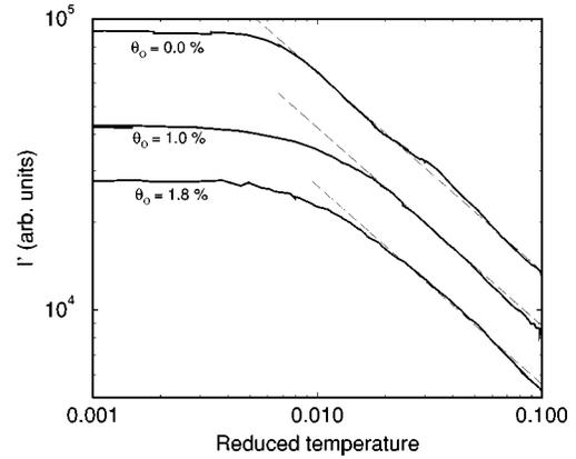
FIG. 10. Derivatives with respect to temperature,  $I'$ , of  $(2 \times 2)$ -2H superstructure spot intensities versus reduced temperature below  $T_c$  after the indicated amounts of oxygen were preadsorbed. The dashed lines indicate a power law with the critical exponent  $\alpha = 0.68$ , which was determined from the oxygen free system.
