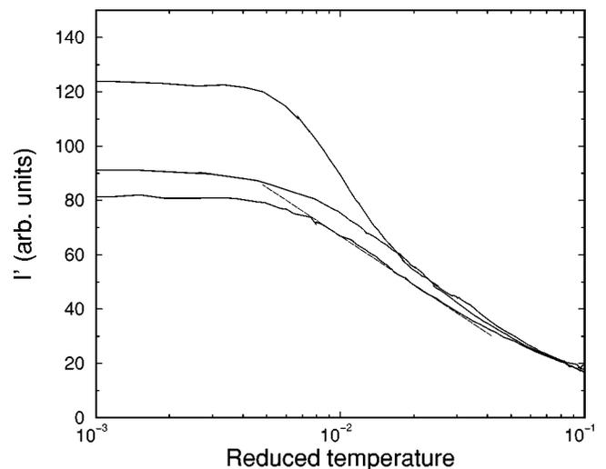
FIG. 11. Semi-log plot of the temperature derivatives of integrated intensities of  $(\frac{1}{2} \times 0)$  superstructure spots with 0%, 0.7% and 1.5% ML of oxygen preadsorbed (from top to bottom). Dashed line corresponds to logarithmic behavior. Leveling-off below  $t < 0.007$  for all curves is due to finite-size effects.
