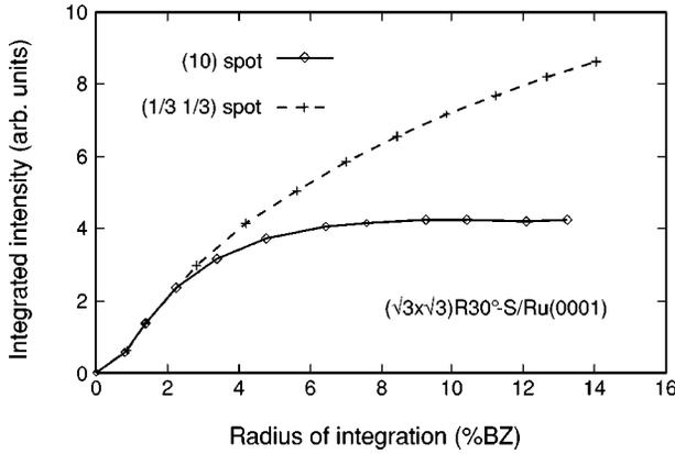
FIG. 12.  $(\sqrt{3} \times \sqrt{3})R30^\circ\text{-S/Ru}(0001)$ : Integrated intensities centered at the  $k_{\parallel}$  positions of the  $(\frac{1}{3}, \frac{1}{3})$  and  $(1 0)$  beams, respectively, as a function of the radius of integration. The radii are measured in units of the diameter of the Brillouin zone (BZ). Measuring temperature was 400 K.
