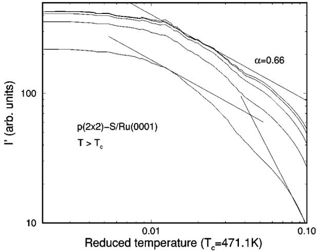
FIG. 7. Log-log plot of the derivatives of integrated intensities,  $I'$ , above  $T_c$  for S/Ru(0001)- $p(2 \times 2)$  measured with the radii of integration (curves from bottom to top)  $K_I = 1.35, 2.7, 4.0, 5.4,$  and  $8.0\%$  BZ. The straight lines in the middle correspond to the power-law behavior found below  $T_c$  ( $\alpha = 0.66$ ). The slope of the straight line drawn in the lower right corner corresponds to a slope of  $-(\gamma + 1) = -2.17$ .
