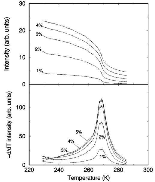
FIG. 3. Top: Temperature dependence of integrated intensities of the  $(\frac{1}{2}, 0)$  superstructure spot in the system  $(2 \times 2)$ -2H close to the order-disorder phase transition for various radii of integration (in units of the diameter of the substrate Brillouin zone). Bottom: Same intensities differentiated with respect to temperature. The critical temperature was determined by the maxima of these curves.
