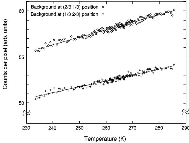
FIG. 1. Temperature dependence of the background intensity of  $(2 \times 2)$ -2H, integrated over a circle of 6% BZ radius, centered at  $K_1$  and  $K_2$  points of the surface Brillouin zone. Intensity increases linearly with temperature as indicated by the straight line. For details of the temperature dependence see text.
