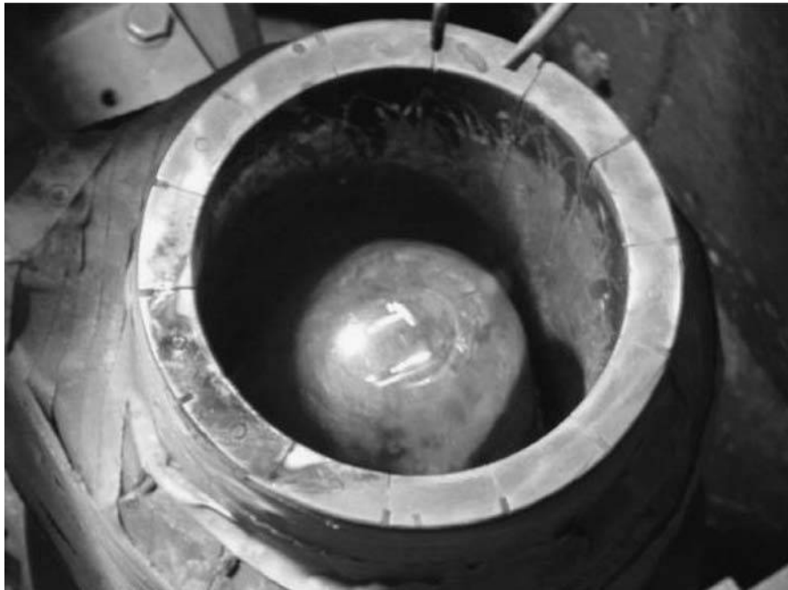
Figure 1. Induction furnace with cold crucible
