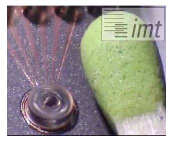
Figure 10. Rotating micro variable reluctance actuator
