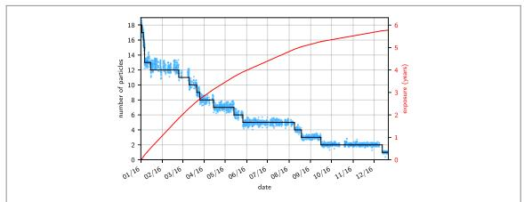
**Figure 4.** Determination of the exposure in the RT. The filtered dip width data as function of the date is shown as blue dots, the corresponding particle number as black line. Each time when a particle is extracted towards the precision traps, the particle number decreases by one. Integrating the time including the corresponding particle numbers yields the exposure, shown as red curve.
