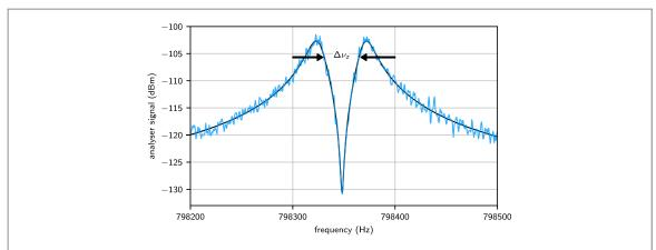
**Figure 2.** Fast-Fourier transform of a time transient signal of the axial detection system with a cloud of 18 antiprotons tuned to the centre of the detector. The width of the short in the noise resonance is proportional to the number of trapped particles. Measured data is shown in blue, the black curve represents the fit to the data. For more information, see text.
