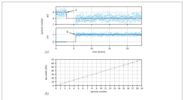
**Figure 3.** (a) Particle numbers obtained from the measured dip widths as a function of time in the reservoir trap (RT) and the precision trap (PT). Extraction removes a particle from the RT (A). The particle is then transported to the PT where it appears on the detector's noise spectrum (B). (b) Measured dip widths as function of particle number. By fitting a straight line to integer numbers as function of the dip widths yields the calibration factor to determine the number of particles.
