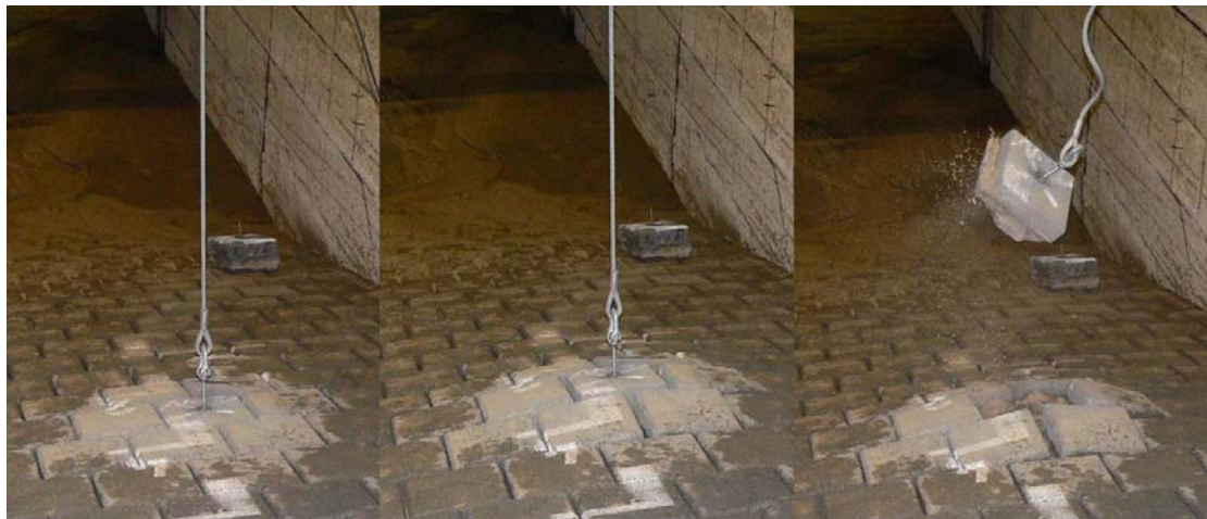
Figure 7. Chronological sequence of a pull out test
