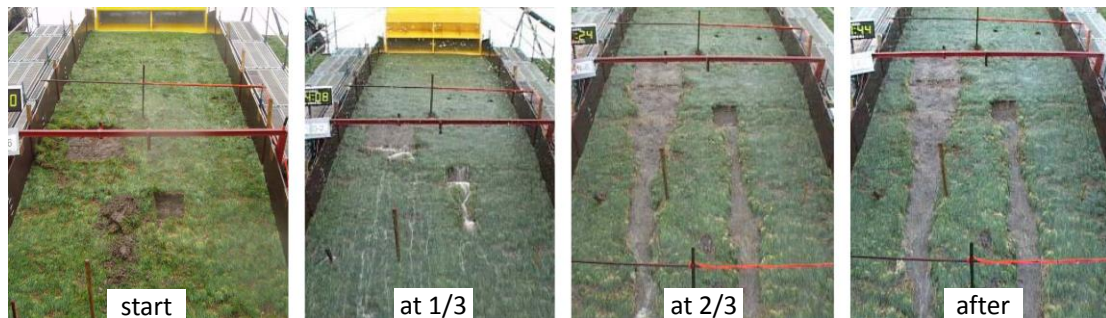
Figure 5. Results of overtopping tests by including initial damages in grass cover and clay layer of the dike (Akkerman et al., 2007).
