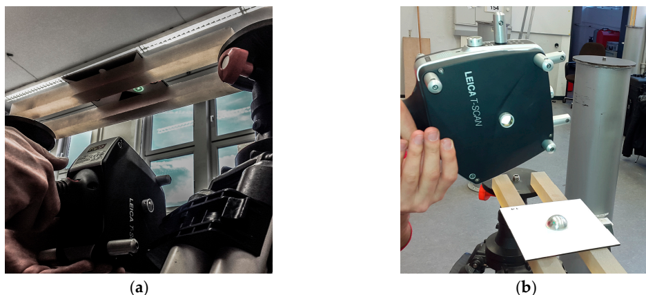
Figure 10. Scan of each targets (a) front side and (b) backside with Leica T-Scan 5 for the determination of the target radius.
