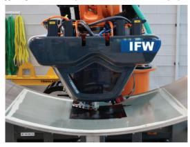
Fig. 3. Laying head with integrated IR camera
