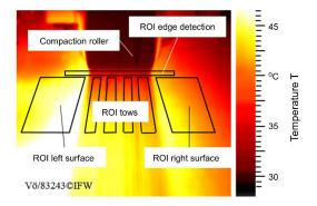
Fig. 2. Regions of interest for the surface inspection by an IR camera
