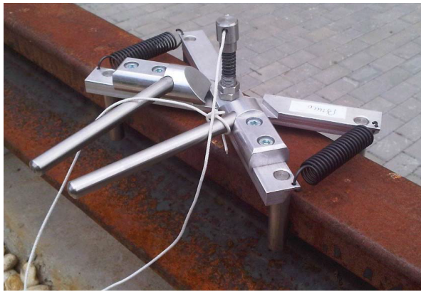
(a) Special rail scissor [8] for the direct measurement of the rail axis mounted on a rail. The reflector is not shown in the picture. (Reproduced with permission from Mr. Vladimír Molčan, Deformation surveying of crane track; published by Mr. Molčan, 2014.)
