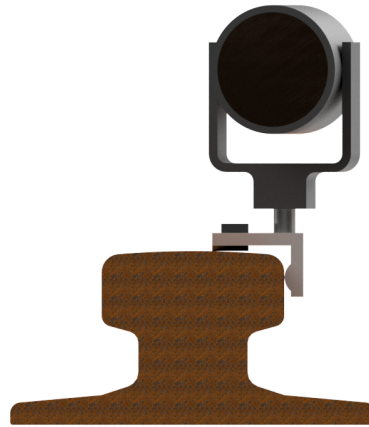
(b) Rail measuring angle with a reflector mounted on a rail. The level can be set vertically with a level. The shown angle is in accordance to [9].
