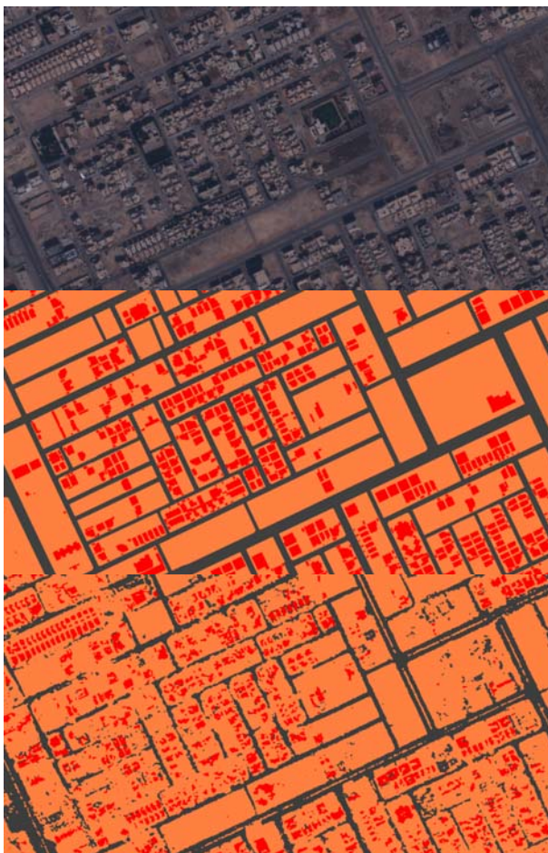
Figure 7: Upper row: GeoEye (left) and Ikonos (right) image. Middle row: Reference label image (red: building; orange: ground, dark: street). Lower row: Classification results, GeoEye (left) and Ikonos (right).
