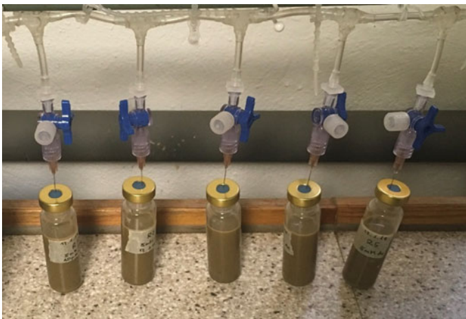
Plate 3.4 Flushing of incubation vials containing soil slurry
