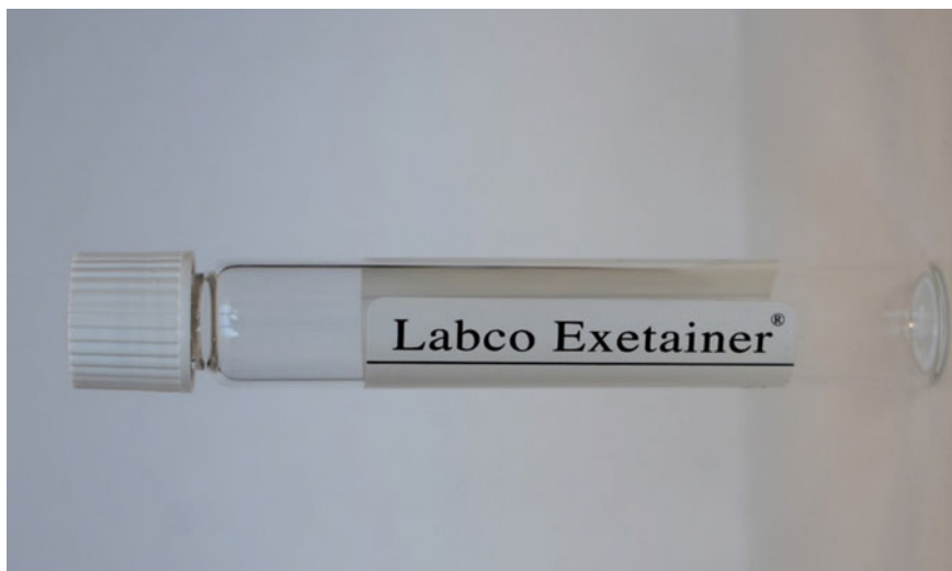
Plate 6.7 Exetainers for gas storage
