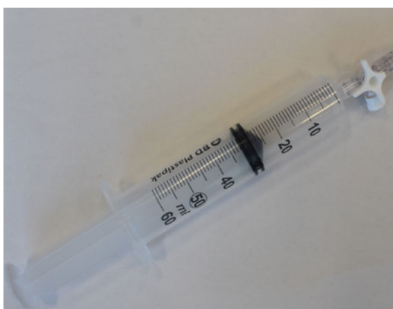
Plate 2.15 Gas collection through a syringe in the field
