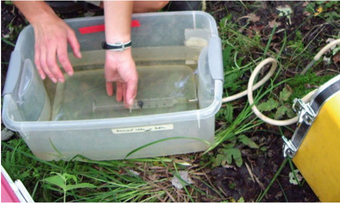
Plate 2.17 Groundwater being sampled from a piezometer tube using a peristaltic pump. Note the syringe is kept under water to prevent any contamination by air while it is being filled
