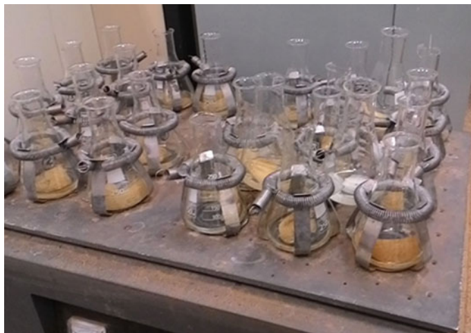
Plate 2.25 Orbital shaker with the Erlenmeyer flasks used for the extraction of \text{NH}_4^+ from the foams coming from the chambers
