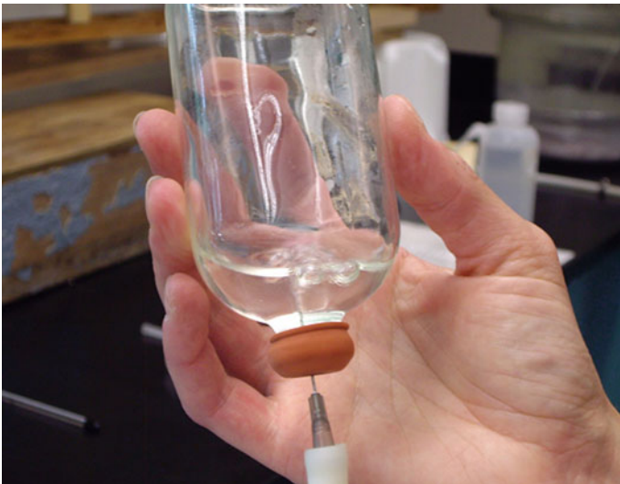
Plate 2.18 A water sample has been previously injected into the serum bottle. Here, the He is being injected, with the bubbles indicating He gas is still entering the serum bottle, once bubbling ceases the headspace will be at atmospheric pressure, the needle will be removed, and equilibration of the water and gas phases can occur
