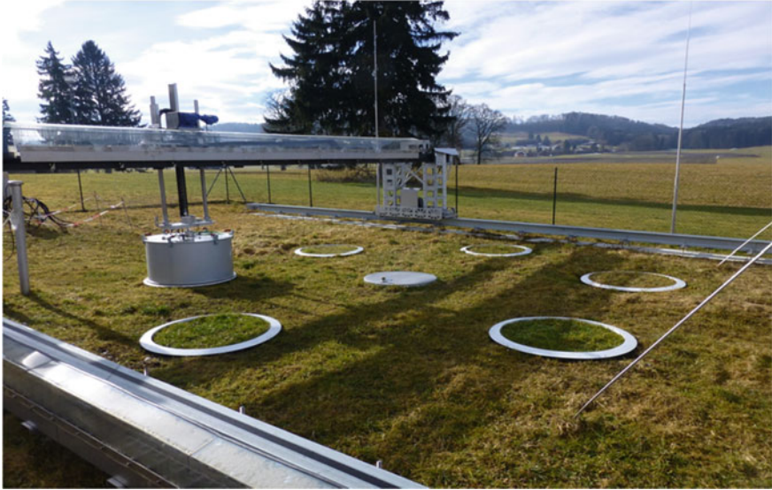
Plate 3.8 Automated GHG flux measurements at a grassland site in Bavaria by the Institute of Meteorology and Climate Research, Atmospheric Environmental Research (IMK-IFU), Garmisch-Partenkirchen, Germany, using a closed chamber robot system in combination with lysimeters. For this installation, undisturbed soil monoliths (1 m diameter, 1.8 m depth) were taken at various locations along a climate gradient and re-installed at a common site. This setup allows to monitor short- and long-term effects of climate change (changes in rainfall and temperature) on ecosystem \text{CO}_2 , \text{N}_2\text{O} , and \text{CH}_4 fluxes as well as on groundwater recharge and leaching of nitrogen compounds ( \text{DON} , \text{NO}_3^- , \text{NH}_4^+ ). Photo: courtesy of Dr. Ralf Kiese, who is also leading this research programme at IMK-IFU, which is part of the German Helmholtz TERENO initiative
