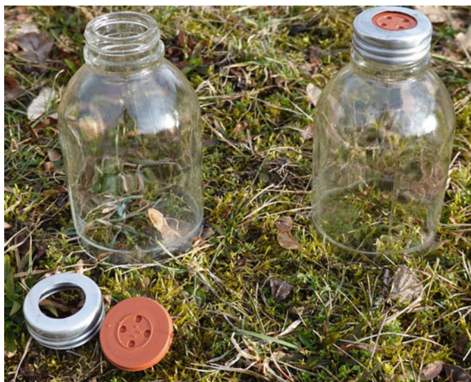
Plate 2.3 Glass chamber consists of only one part (Šimek, personal communication) for measuring GHG emission from pasture soils
