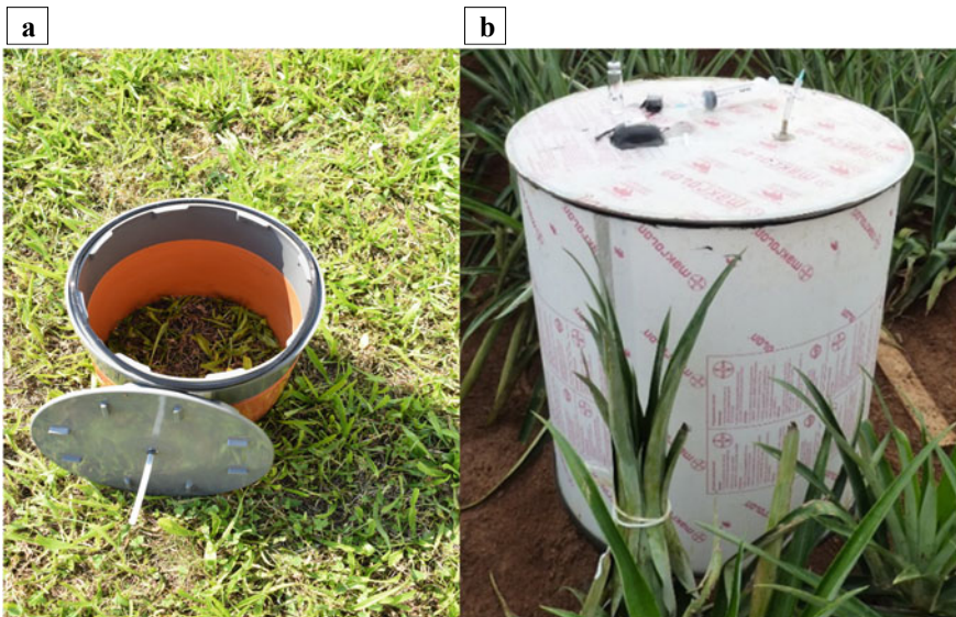
Plate 2.2 Plastic chamber made up of two parts: vessel and lid for measuring greenhouse gas emission from a pasture soil and b arable and vegetable croplands
