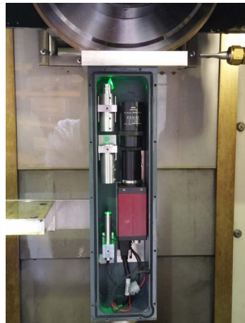
Figure 10. Installation of concept C in the manufacturing machine.
