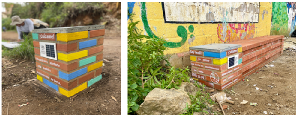
Figure 7. Sensor protections as small seats or benches made out of bricks, supplemented by short inscriptions and bright colors.
