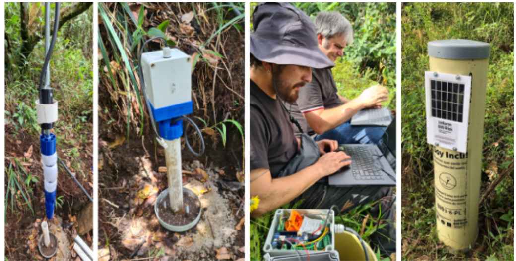
Figure 4. Photos of the installation of the measurement system in Bello Oriente in 2022. (Left): Installation of a subsurface probe with a measurement node on top. (Right): low-cost sensor enclosure in a remote location.
