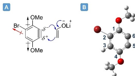
Figure 4. Regioselectivity of aryne [2 + 2] cycloaddition. A) The -I effect of Br on the triple bond. B) The optimized calculated structure of the benzene intermediate at B3LYP/6-31 + (d,p) level of theory.
