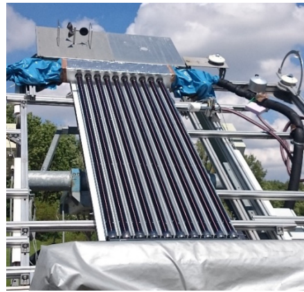
Figure 4. Measurement of the zero-loss coefficient and the IAM behavior on a solar tracker.
