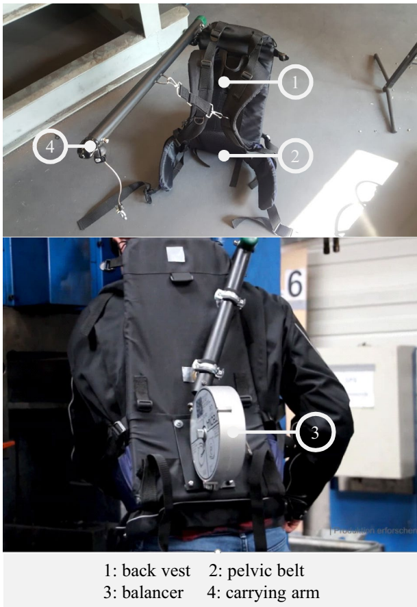
Fig. 7 Support frame for facilitated guidance of forged parts
