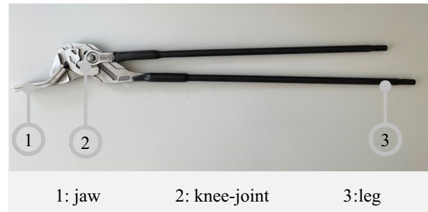
Fig. 5 Structure of some knee-joint forging tongs
