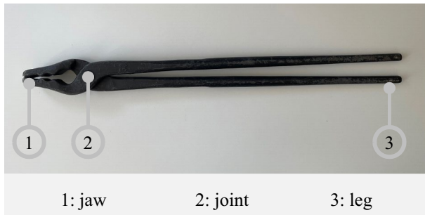
Fig. 3 Structure of some conventional forging tongs
