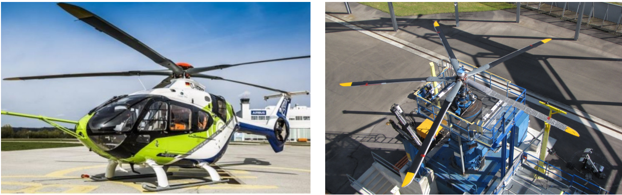
Figure 2.7: GRC1 prototype rotor on the Bluecopter™ demonstrator (left) and whirl tower (right), Kus et al. [124].
