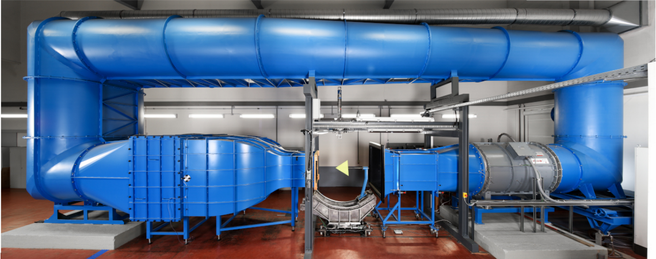
Figure 3.2: One-meter wind tunnel Göttingen (1MG) after its refurbishment in 2014/15, configured with an open test section.
