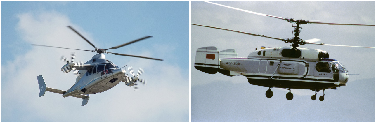
Figure 1.3: Airbus X 3 technology demonstrator, note the auxiliary wings and propulsive rotors (left, adapted from [56]), Kamov Ka-32 “Helix” helicopter, note the two coaxial main rotors (right, adapted from [155]).
