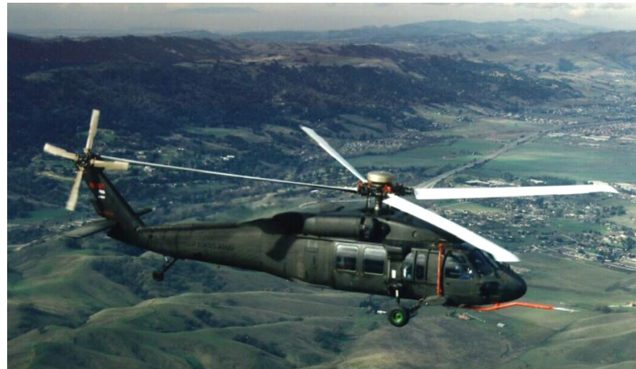
Figure 2.22: Test helicopter of the UH-60A Airloads Program flying with an instrumented rotor blade, note the telemetry system on top of the rotor hub, Ref. [123].
