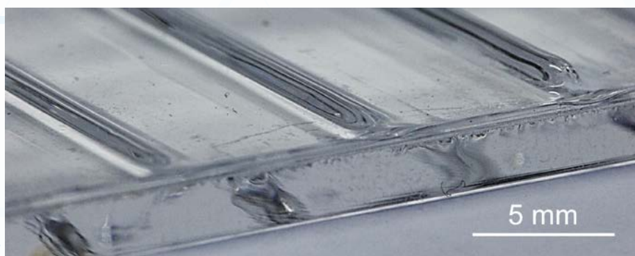
Printed transparent fused silica structures consisting of one, two and four layers (from left to right) without boundary layers.
