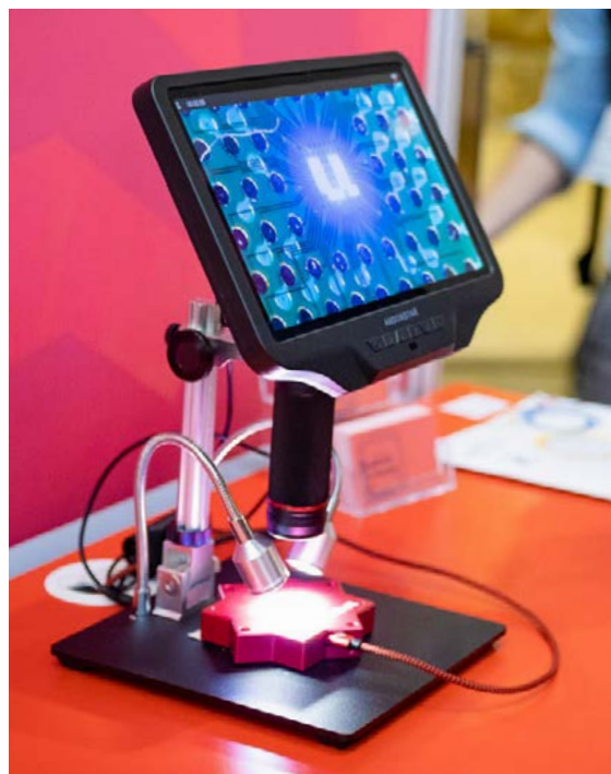
A micro-LED platform playing a fast animation with several thousand frames per second is shown at a trade fair. The demo showcases the current status of the micro-LED arrays as a versatile platform for individual light projection with highest modulation bandwidths and brightness.
