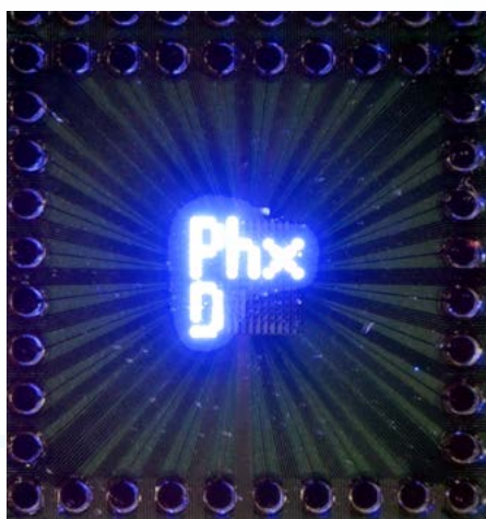
Micro-LED array integrated onto a printed circuit board during operation in full-light emission mode (left) and during display mode showing the letters "PhxD" (right). The pixel size is 30 micrometres, comparable to smartphone displays, but with much brighter light and a faster switch-on time. In combination with advanced colour converters, new mass transfer technologies are needed to accomplish even smaller and multicolour pixels. We develop the manufacturing processes required to realize micro-LED modules, focusing on reliability, high throughput and cost-effectiveness.
