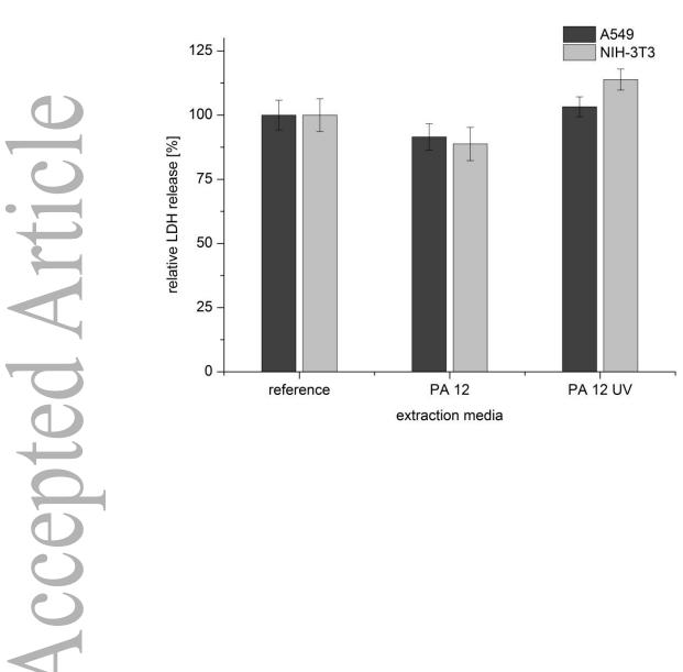
**Figure 5:** Relative LDH-release in the supernatant without cell lysis. These measurements are used for determination of cell death. The LDH-release in the supernatant is caused by the loss of membrane integrity of the cells and indicates necrotic cells. Both cell strains were cultivated in 3D-printed replicas of a 24 well plate, as well as in the standard well plate as a reference. The shown data are an average of four parallel experiments (error bars indicate the SD of the experiments).
