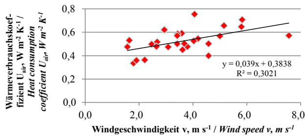
Heat consumption coefficient for air exchange ( $U_{air}$ ) through leakages as a function of wind speed, double glazing (screens open) (15.12.2011 - 12.01.2012)
