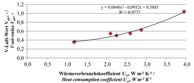
$V_{air}$ -value ( $V_{air}$ ) as a function of the heat consumption coefficient ( $U_{cs}$ ), mean values of measurements with double glazing, double glazing with day screen, double glazing with two screens and double glazing with three screens
