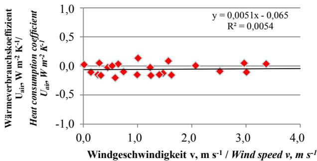
Heat consumption coefficient for air exchange through leakages ( $U_{air}$ ) as a function of wind speed, double glazing and three thermal screens (mean values from 22 pm to 5 am)
