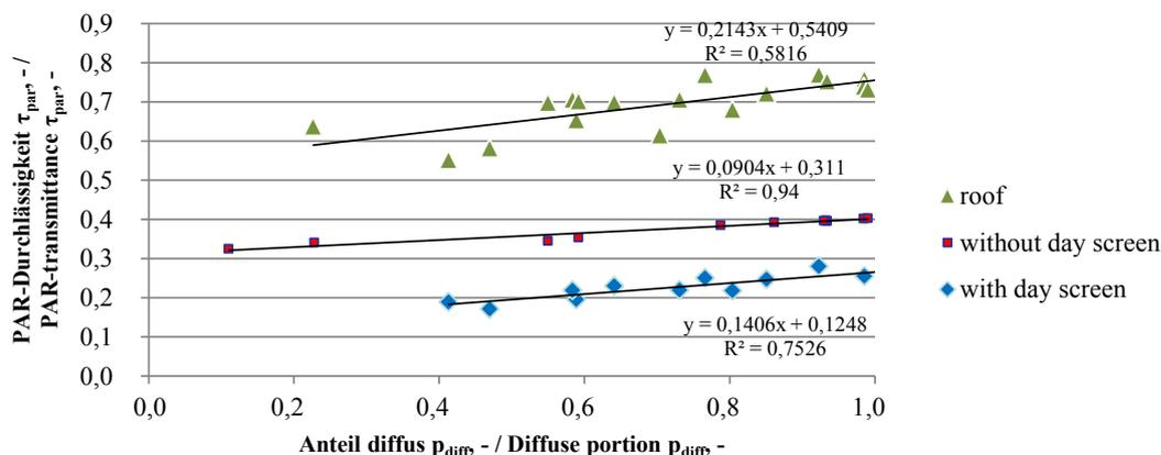
AR-transmittance (par) of a greenhouse north-south orientated, roof (above the screens), at the height of plant canopy with and without day screen (08.02.-03.03.2012)
