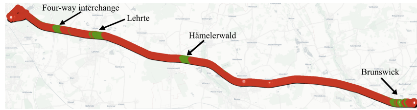
Figure 3.15: Map indicating availability of carrier aggregation (green = available, red = not available). In our measurements, carrier aggregation was only available close to populated areas or an interchange where more traffic is expected. Map data © OpenStreetMap contributors, CC BY-SA [26].
