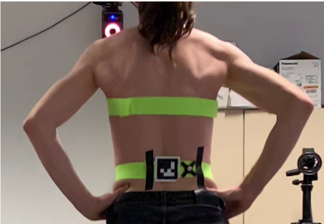
Fig. 2. Marker configuration in the lower back region, attached to an elastic strap. Next to the ArUco marker, the motion capture marker can be seen on an X-shaped touch fastener. An equivalent marker assembly was attached to the chest of the subject using the second strap.
