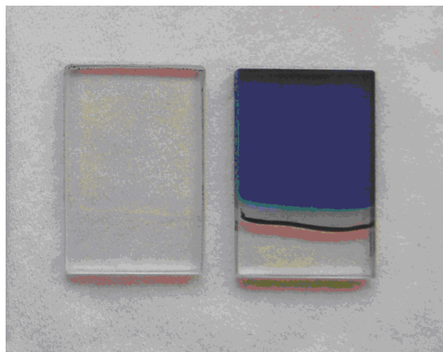
Figure 11. Mesoporous ITO film prepared using PIB-PEO 3000 on glass (left) and FTO-coated glass (right) after electrochemical deposition of PB.
