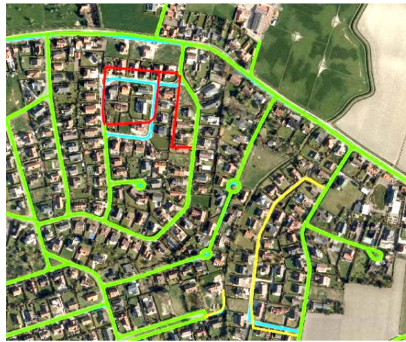
Figure 9: MMV successfully detects changed roads within a residential area (MMV outcome: correct = green, incorrect = red, undecided = yellow, reference = blue)
