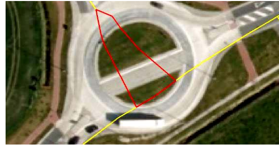
Figure 6: Redeveloped traffic circle identified by grassland detection (rejected roads = red, no decision = yellow)
