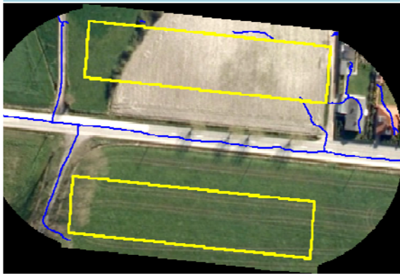
Figure 1: 2D line extraction result (blue) and region mask (yellow) for computing entropy E
