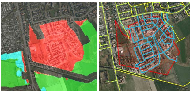
Figure 8: Redevelopment detection; Left: no contradictions to the database = green, irrelevant contradictions = blue, contradicting regions denoting impervious surface = red; Right: current road data = yellow, roads required to be updated = blue, methods outcome = red
