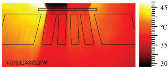
Fig. 9. Tow 3 and 4 winded around the compaction roller
