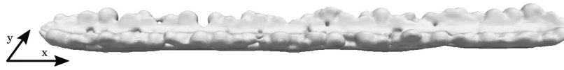
Figure 6.26. Side view of the melt pool under the influence of gravitational and buoyant forces according to equation 3.29.
