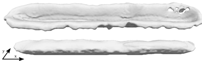
Figure 6.30. Side view of the melt pool under the influence of gravitational, buoyancy and surface tension forces, the Marangoni convection and the recoil pressure. Top: temperature decreasing surface tension; bottom: temperature increasing surface tension.
