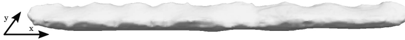
Figure 6.27. Side view of the melt pool under the influence of gravitational, buoyant and surface tension forces.
