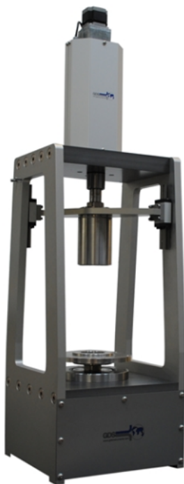
(a) Interface-Shear-Tester der Firma GDS Instruments, Hook, Hampshire, United Kingdom [64]
