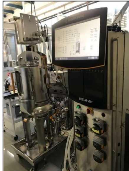
Figure 19 : Single use stirred tank bioreactor with a maximum working volume of 50 L
