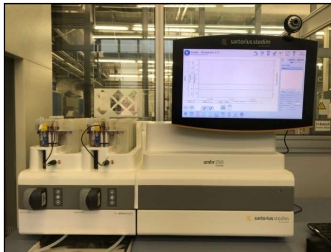
Figure 22: Microbioreactor with maximum working volume of 250 mL (AMBR 250 )
