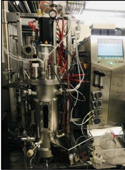
Figure 16: 10 L stainless steel bioreactor used for scalability test
