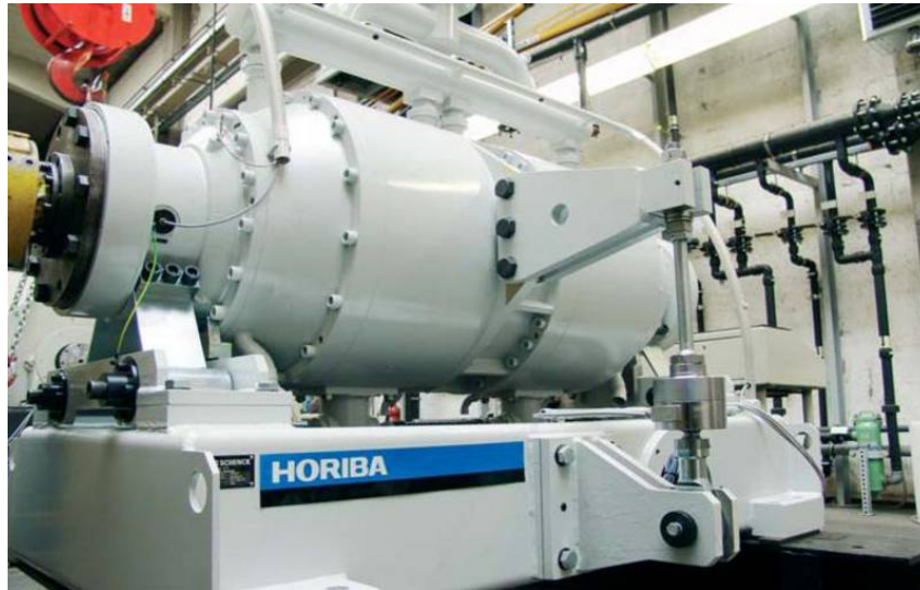
Figure 2.2: The DT type hydraulic dynamometer from HORIBA [50]
