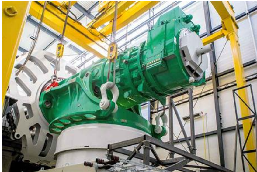
Figure 1.1: Adwen test campaign in DyNaLab [9] at Fraunhofer IWES
