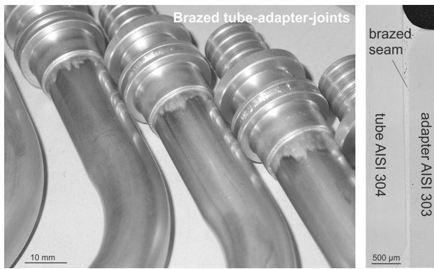
Fig. 8 Stainless steel components joint with copper braze at 1100 °C in a conveyor belt furnace under SiH 4 -doped nitrogen. Right: optical microscopy image of a cross section from a joint
