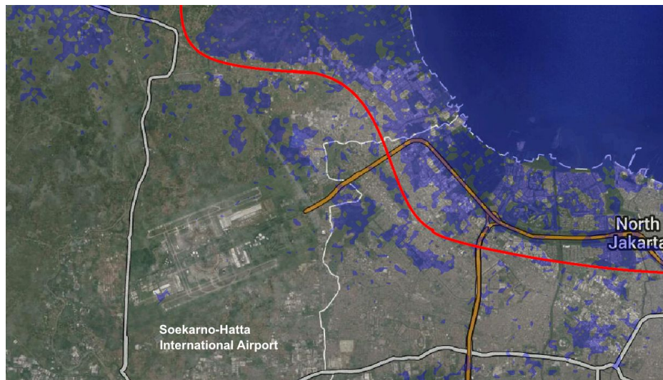
Fig. 12 Static flooding simulation of North Jakarta, airport area [map: Google Maps; topographic data: SRTM].
