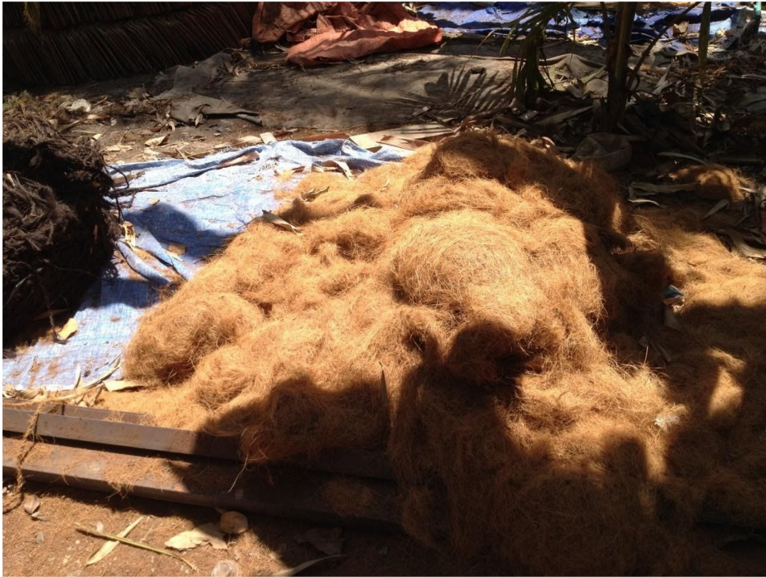
Fig. 5 Extracted coir fibers, the raw material for coir products such as geotextiles, © David 2014
